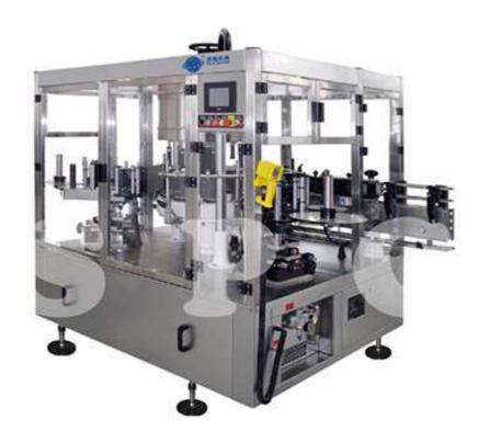
This machine is fully automatic rotary self-adhesive labeling machine. Used for different industries for beer, white spirit, seasoning, soft drink, mineral water, cosmetics, cans and others. It has the advantages of humanized design, flexible and convenient adjustment, easy to operate, low speed and large torque. Clean labeling environment, high stability, It's the necessary labeling machine for the company to upgrade their product and quality.
