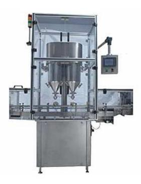
SBAF-D-100 Automatic Double Head Auger Type Dry Syrup Powder Filling Machine is a compact model used for filling Dry Syrup Powder in bottles.
