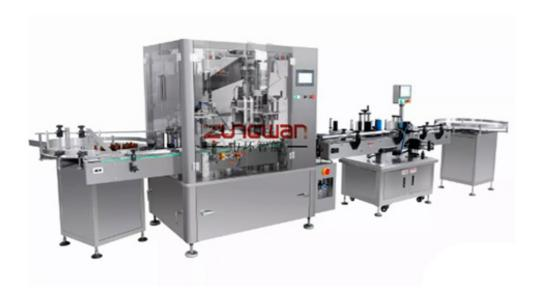
This machine has the functions such as automatically screw type bottle feeding, bottle detecting (no bottle no filling, no bottle no cap feeding), filling, cap feeding and capping automatically.
