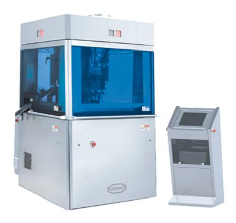
Cadmach presents its C-Series, Single Rotary Tablet compression machine which is a fully automatic, high speed, interchangeable turret design machine and with technology incorporating Industry's requirements for performance & quality. This is highly suitable for Medium Scale Production. The C 200 Pill Compressor Machine is offered in 30D, 36B & 43BB Turret Configurations
