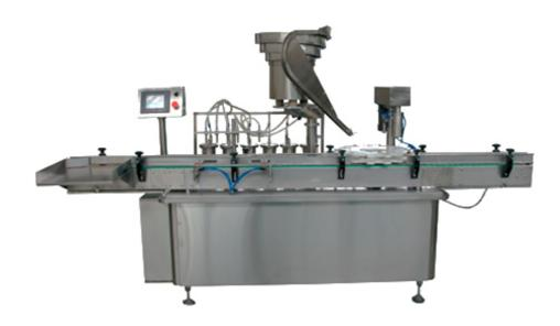
This machine is the main filling equipment of the oral liquid production line, which is Mainly applied in the filling, covering and sealing of the 30 - 500 ml bottles.
