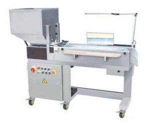
The product flows from the feed hopper into a vibratory chute where a perforated screen eliminates coarse dust and chips, which are then collected in a collecting container.
