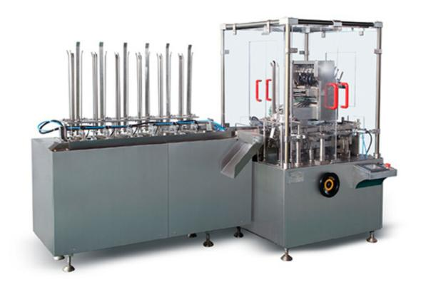
This machine can pack Granule bag, Condom, Aluminum strip, plaster, coffer sachet, facial mask, blister and so on.
