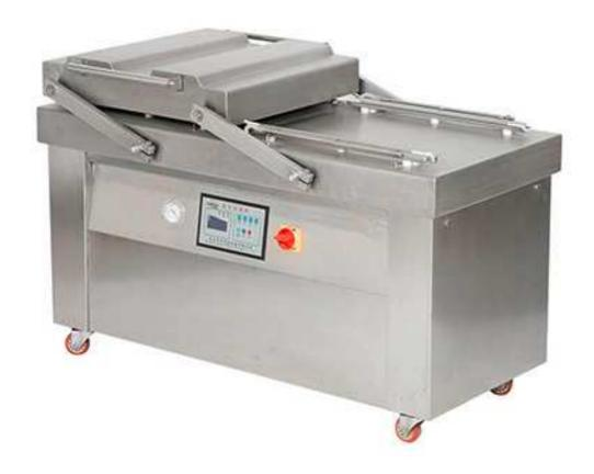
DZ600/2S vacuum packing machine sealing line length is 600mm, equipped with 3 well-known vacuum pumps, LCD screen showing vacuum time and sealing time, can be set the relevant parameters according to the product, is one of the high cost performance equipment in the double room vacuum packing machine.
