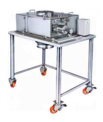
Oscillating granulator is used for gentle homogenization, size reduction, grading and sieving of dry, sensitive powders and granules in pharmaceutical, chemical and food industries.
