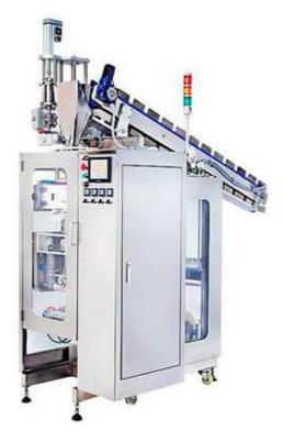
TD-V25L VFFS Packaging Machine for Liquid uses servo-driven film roll. Color touch screen operator interface, tracking automatically adjust depending on length of the bag packaging film printing position.
