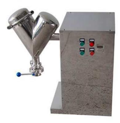
This machine is suitable for mixing more than two kinds of dry powder and granular materials in pharmaceutical, chemical, food and other industries. The mixing cylinder of this machine has unique structure, high mixing efficiency, no dead Angle, made of stainless steel material, internal and external wall polishing treatment, beautiful appearance, uniform mixing, wide applicable surface, and can be matched according to the requirements of users.
