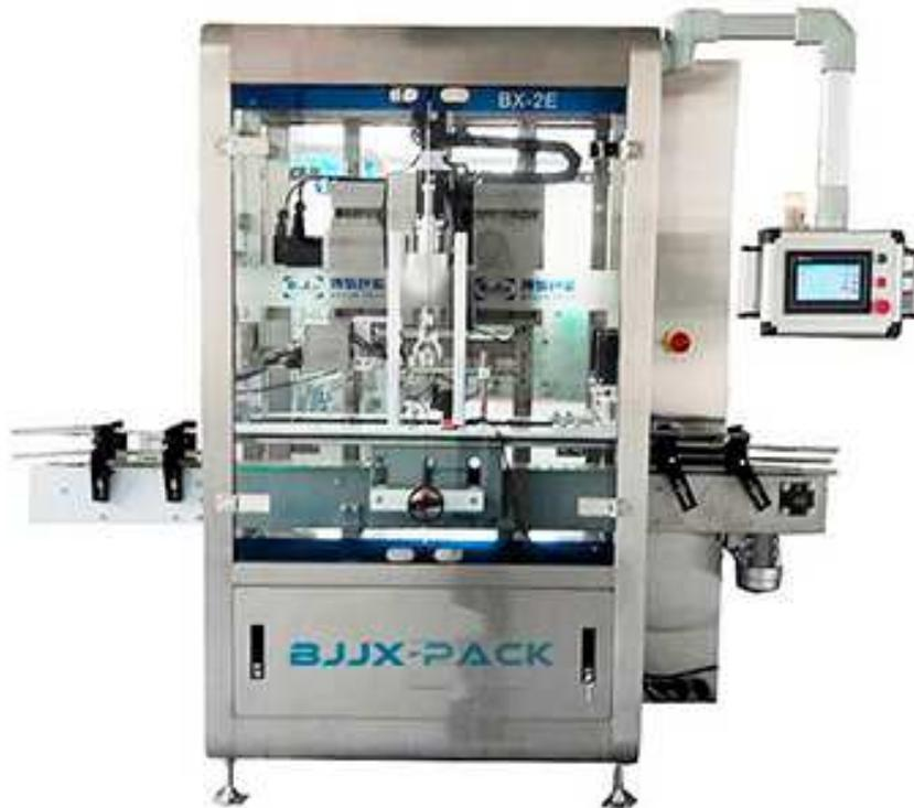
The single head capping machine has good practical applicability for various cap. And only change cap screw head, and it doesn't hurt cap.
