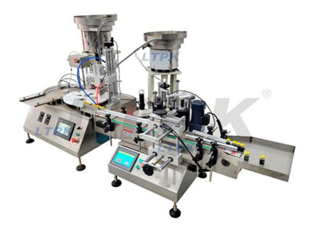
This filling capping machine is designed for the vial, this is a custom made machine, we can custom it for a variety of small plastic or glass bottles. It can sort bottles, fill liquid into bottle, tighten bottle caps. It is also equipped with cap vibratory bowl sorter which can feed bottle caps automatically. And equipped with a desktop round bottle labeling machine to form a production line, saving production labor.
