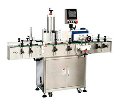
This Automatic Labeling Machine can equip with bottle filling machine, it is economical, self contained, easy to operate, equipped with auto teach programming touch screen. Built in microchip storing different job setting makes fast and easy changeover.
