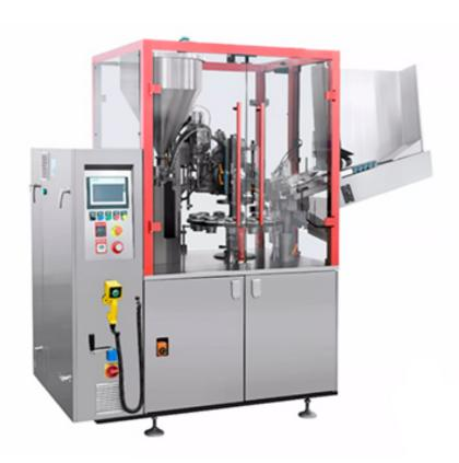
The machine is automatic for its finding mark, sealing, printing lot number and tube out automatically. Adopts inner heating system by using Swiss heater "LEISTER", by blowing hot air to inner wall of the tube to melt the plastic and then printing insection and lot number. toe index adopts precise cam, precision and placidity. toe index motor by using transducer to adjust speed, users can adjust running speed.
