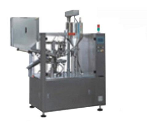
This NF-100A fully automatic tube filling and sealing machine is applicable to processing the plastic and aluminum tubes.
