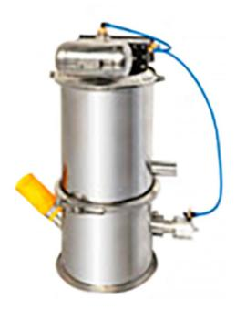
The QVC automatic vacuum conveyor utilizes compressed air to realize material conveying. Requiring no mechanical type vacuum pump, the compressed air passes through the vacuum generator of the vacuum feeder, thus high vacuum environment is created. Thanks to the high vacuum, the material layering is fully avoided, ensuring the uniform mixing of the material.
