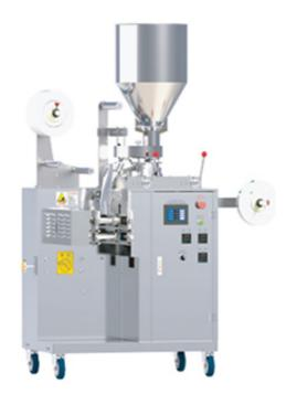
YS-11 Tea bag with thread and label packing machine is suitable for packing of steeping products automatically. Such as broken tea, medicinal tea, coffee, plant minced. All the works of bag making, measuring, filling, sealing, cutting and counting can be done automatically, at the same time, wearing, cutting the thread with cutting and sticking label one by one.
