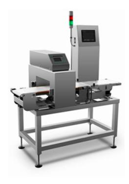
Metal detector supplier is used to detect metal on food production line before or after packing to make sure safety of finished food package.
