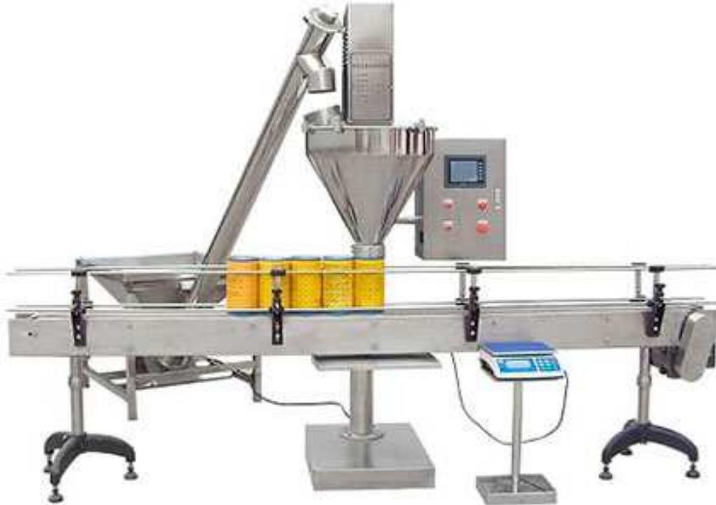
Automatic single head linear powder filling machine of model VTOPS-PSH-01 is an economic type auger filling machine. The containers are automatically position, automatic filling and automatic transferring.
