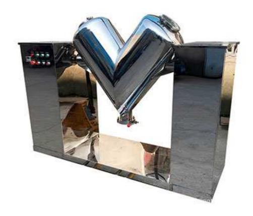
V Mixer Machine is suitable for mixing dry powder or particles. The machine is a Stand Mixer and occupies little space. The V-shaped rotates under the drive of the motor, and the material in the barrel is constantly gathered and dispersed to get a uniform mixture. The powder Mixing Machine is simple in structure, easy to operate and widely used V Series Mixer.
