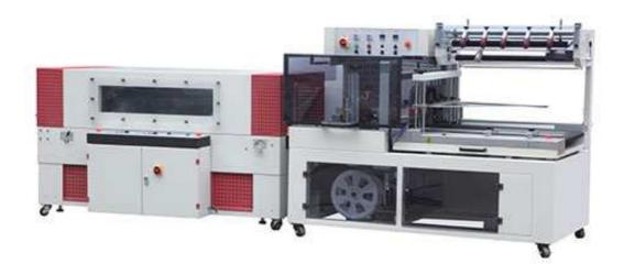
This L type sealer machine is widely used in foodstuff, drinks, printing, pharmaceutical, floor, hardware and other industries shrink packaging. It is suit POF, PE, PVC and other packaging material
