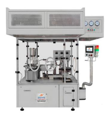
HMPL Sterile offers the cutting-edge ACCUFILL LPFS COMBO 60-OA – a high-performance Nested Pre-Filled Syringe, Cartridge, and Vial Filling & Stoppering Machine designed for 0.1 ml to 5 ml pre-filled syringes. Operating at 1 ml, this advanced system delivers an impressive output of 40 to 60 devices\\* per minute with precision and efficiency.
