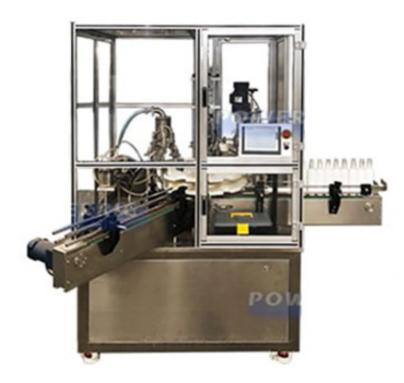
A vial filling machine is used for filling and packaging sterile liquids, powders, and other pharmaceutical products into vials. The machine automates the process of filling, capping, and labeling vials, which is crucial for maintaining the sterility and integrity of the products being filled.
