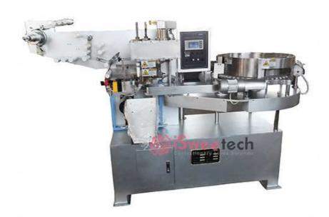
This is the newly developed wrapping machine specially designed for ball-type lollipops. It is high speed and reliable function.
