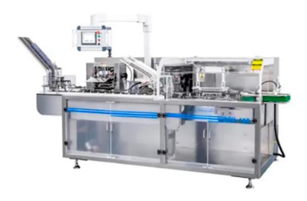
The DZH-120 Horizontal Cartoning Machine is capable of reliably loading items with a stable or regular shape within a certain size range into cartons of specific specifications and sealing the cartons for delivery. It is suitable for carton packaging of various medicines, food, cosmetics and other related industries.
