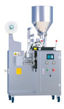
YS-10 Tea bag with thread packing machine is suitable for packing of steeping products automatically. Such as broken tea, medicinal tea, coffee, plant minced. All the works of bag making, measuring, filling, sealing, cutting and counting can be done automatically, at the same time, wearing and cutting the thread.
