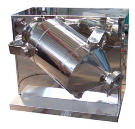
During running, as the mixing vat is able to make multidirectional operation, Such as level movement, rotation, turning and other complex movements. This speeds up the flowing and diffusing actions of material in mixing process, which is avoiding gravity segregation or accumulation phenomenon of general mixers caused by centrifugal action. Therefore, this machine has favorable mixing efficiency.
