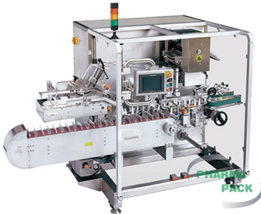
The LFBI-12 is a versatile cartoner which is ideal for the pharmaceutical and nutraceutical industries. With speeds up to 120 cartons per minute, cartons are automatically transported by a toothed conveying belt. A rotary encoder monitors linear movement which allows for the handling of even the most difficult to open cartons with ease. The rugged stainless steel construction will fit seamlessly in your.
