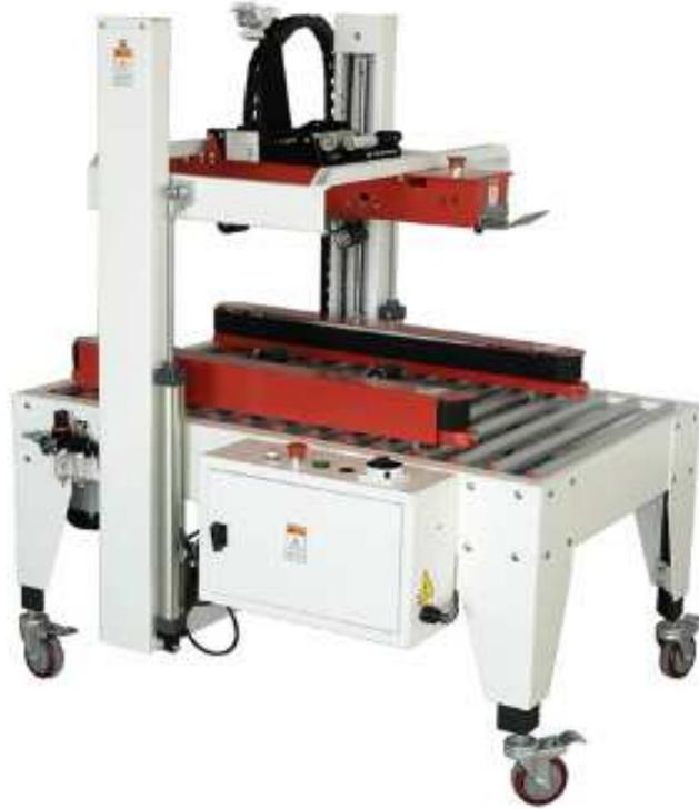
This machine's quality is better than so many carton sealing machines in Turkey. It is designed for saving time, and working with fewer workers. This machine seal the carton without any adjustment. Only thing you have to do is put the carton in the front of machine. This machine automatically adjust the sizes and seal it.
