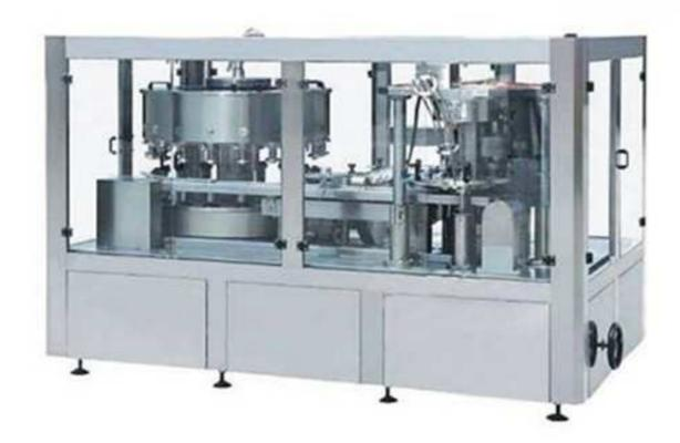
The carbonated drinking filling machine could be separated to 3 modules. The height of the bottle-out conveyor is adjustable. Bottles are conveyed to rinse, filler and capper through star wheel and conveyed out finally through bottle-out conveyor. Equip with alarm device for bottle block, bottle absence, cap absence and overload. The machine meets the national food hygienic standard, with high automation and easy to operate.
