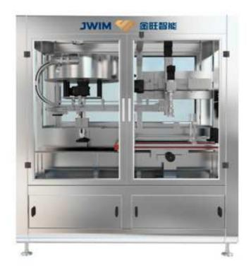
FXG-1H full-automatic following type capping machine is composed of cap conveying mechanism, capping mechanism, moving module, bottle conveying mechanism and control system. The machine has simple structure and convenient adjustment. The product completes the capping action in the process of moving, which is different from the normal capping machine that needs to stop during capping.
