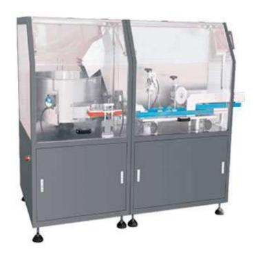
High Speed Bottle Unscrambler is the latest generation mechatronic equipment (consists of bottle lifting device, arranging device and the mainframe). Generally unscrambler in current market is only available to arrange round or rectangular bottles. But the latest machine can solve the problem and applicable to various size of bottles.
