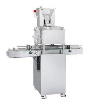
The CDR-3A orbital electronic pill counting machine is equipped with an original orbital feeding structure, which has the superior performance of stability, low noise, and smooth delivery of pills. At the same time, it is made of silicone material to ensure the safety of the contact surface with the material and avoid the shortcomings of tablet damage caused by traditional vibrating discharging.
