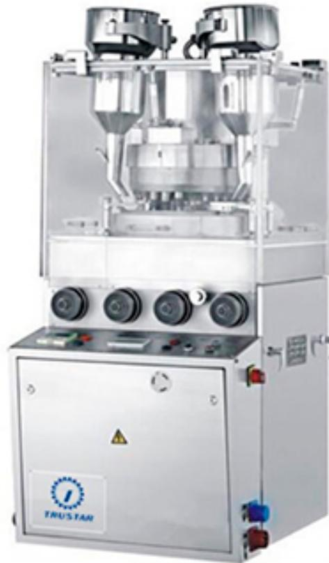
The machine is one kind of single side rotary tablet press machine which can press granular materials into round shape tablets, irregular tablets or double-side engraved tablets. This machine is mainly used in pharmaceutical, chemistry, foodstuff, electronic industries.
