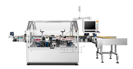
Double Head Rotary Labeling Machine is ideal for small round glass bottles and tubes, it is widely used in pharmaceutical, daily use chemicals, food, beverage, and other industries. The labels can be transparent or opaque, polypropylene or paper, etc.
