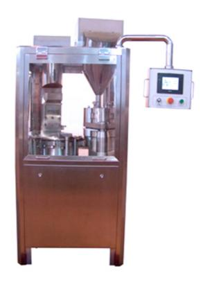
This machine is an intermittent motion and hole plate type filling fully automatic capsule filling Equipment.
