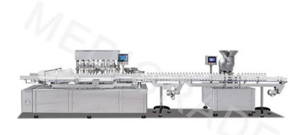
The machine is a straight line intermittent full servoing filling machine. The large dose solvent bottle enters the synchronous belt through the bottle plate and completes the filling and plugging of the liquid in the process of intermittent transmission, and sends it to the downstream equipment or out of the bottle storage plate.
