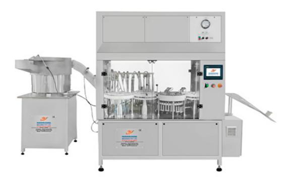
Pre-Filled Flush Syringe Filling and Capping Machine with Reverse System - Top/ Bottom Filling Technology with Leak Proof Cap Sealing System Fill 3 ml to 20 ml volume flush syringes with 80 to 120 syringes per minute.
