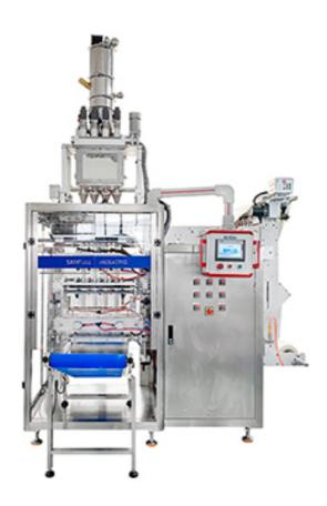
We offer 4-12 lanes four sides sealing sachet packaging machine with the capacity of making 100-540 sachets per minute. is suitable for liquid, powder and small particle, like ketchup, coffee powder, sugar, engery drink, juice, etc.
