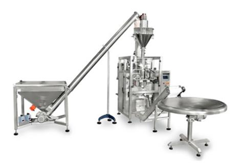
It adopts PLC control with Siemens color touch screen and stable dual-axis high-precision output. Bag making, measuring, filling, sealing, coding, bag cutting and other processes are completed in one go; Using a double belt servo to pull the film: the film pulling resistance is smaller, the packaging bag is well formed and more beautiful, and the belt is not easy to wear.
