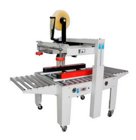
FXJ-5050A are operator fed and designed for heavy duty applications. These machines are reliable, cost-effective and durable providing savings to your production process. More importantly, these machines provide a professional looking seal. The FXJ-5050A Carton Sealer with Easy Manual Carton Size Adjustment has a 2-belt design. The machine comes complete with infeed/exit conveyors, casters, power cord, and plug.
