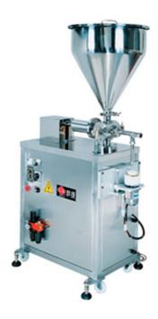
The ointment filling equipment is semi-automatic volumetric filler for high cohesion material such as gel, cream and etc.
