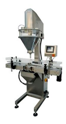
Pneumatic bag clamper and platform equip with load cell to handle two speeds filling as per preset weight. Featured with high speed and accuracy weighing system to guarantee the high packaging accuracy.
