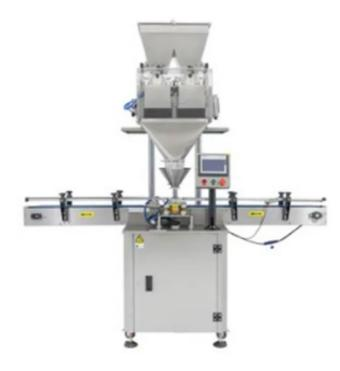
This machine is mainly suitable for weighing all kinds of small granular items in the assembly line.
