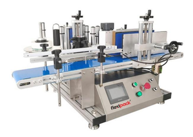
Table top labeling machine is suitable for a wide range round bottles labeling needs, and has high quality and efficiency. It adopts the whole high-grade stainless steel and high-grade aluminum alloy, labeling head using high-speed servo motor to ensure the accuracy and speed of labeling; all the optoelectronic systems are also used in Germany, japan and Taiwan imported high-end products, PLC with man-machine interface control, simple operation clear.
