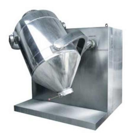
Multi-directional Mixer is a novelty material mixer. The mixing vessel moves in multi-direction. When the driving shaft rotates, the vessel will be in translational and rotational motions under the action of universal joints. Hence, the materials inside the vessel are in three-dimensional compound motions which are in axial, radial and toroidal directions.
