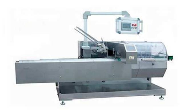
Carton packing machine is especially suitable for bag and bottle products with large specifications.
