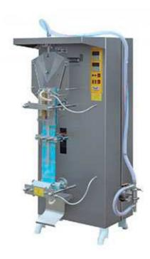
SJ-2000 Liquid packing machine widely used to pack milk, soybean milk, sauce, vinegar, yellow wine, all kind of drink with film. The whole process can be accomplished automatically, such as ultraviolet sterilization, bag figuration, date printing, quantitative filling, enveloping, cutting, counting, and so on. The temperature of heat-sealing is controlled automatically, the production is beauty and fastness, the machine adopts stainless steel shell, and the sanitation is guaranteed.
