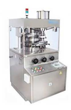
TabXpress-PUV Tablet Press Machine is used for production of simple and precise tablets from powder in Pharmaceutical and relevant Industries.
